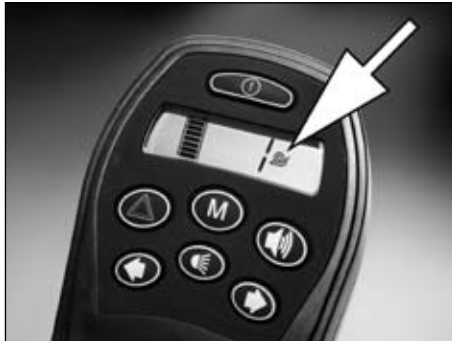
Fig. 24 Snail symbol indicating creep speed
