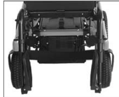
Fig. 11 Footplates flipped up
