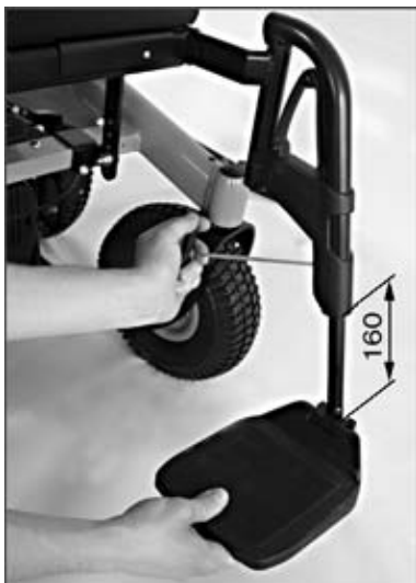
Fig. 10 Adjusting the lower leg length
