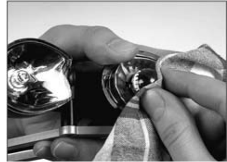
Fig. 28 Replacing the direction indicator lamp
