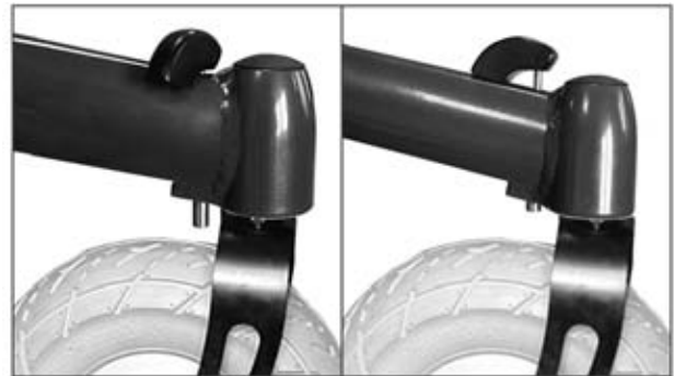
Fig. 31 Caster swivel lock engaged and released
