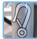
If the wheelchair must be lifted with an articulated crane, to hurdle obstacles, you must not use spots other than the 4 marked with a hook sticker as shown here.
