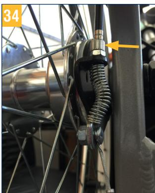
To achieve an optimal braking effect, the braking force is adjusted with the adjusting screw.
