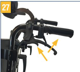
To park, the brakes are locked on both sides by pushing the brake lever. Then push the locking lever on the brake down so that it locks the brake lever.
